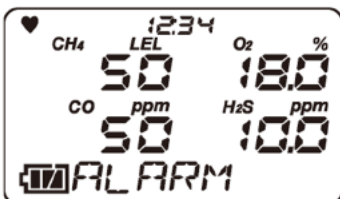
Second alarm setpoint display
